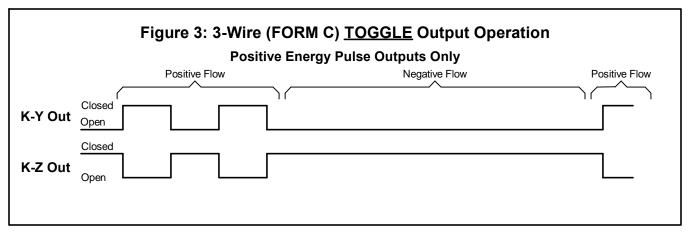
In Signed mode, with a Form C output mode selected, the K-Y and K-Z output pulses represent positive (or kWh Delivered) energy; Negative (or kWh Received) energy is ignored.
